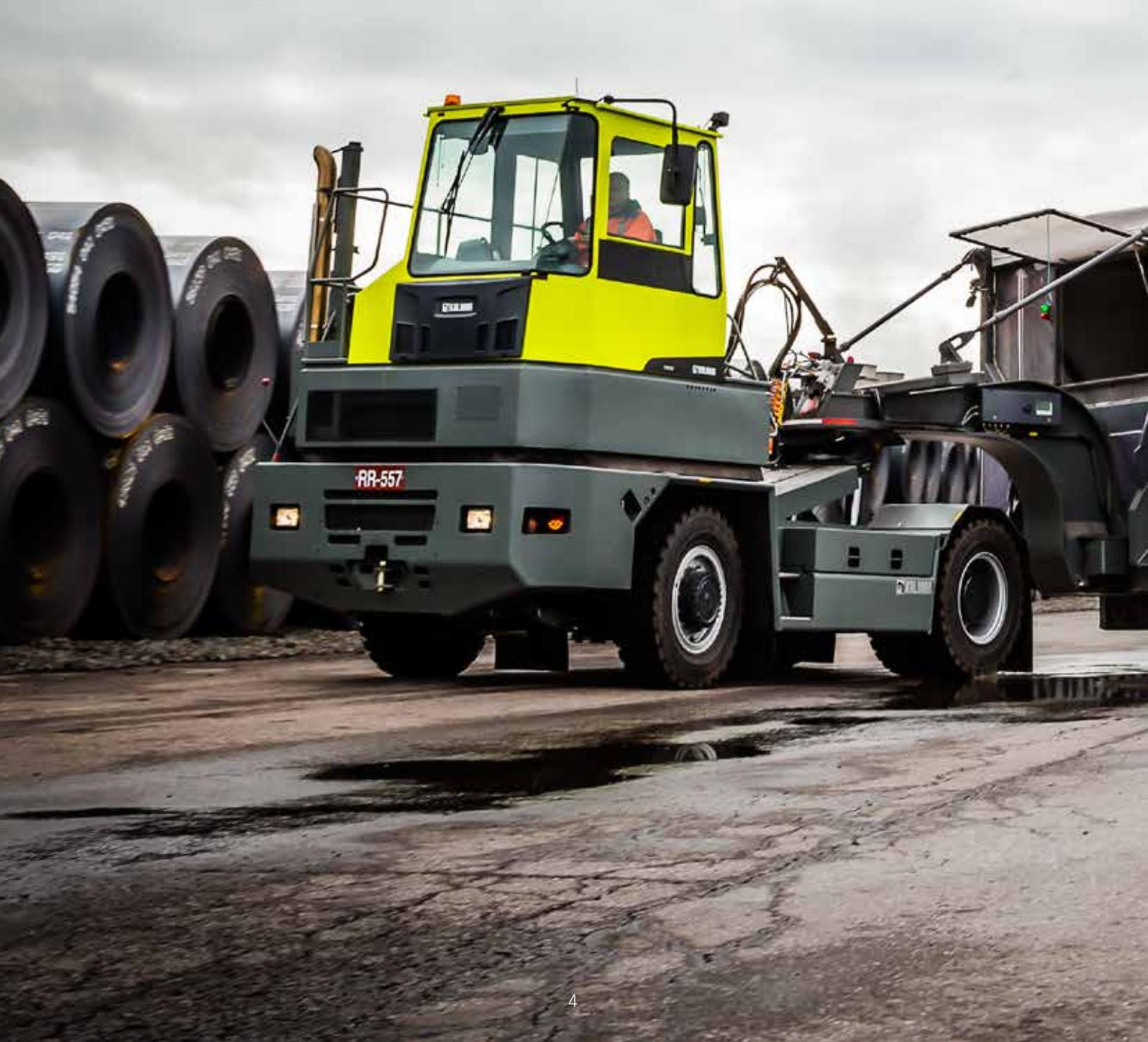
There's also autostop after adjustable idling time to protect the power line, and a long list of other features. The CAN Bus technology provides a flexible platform for lifting height limiters and auxiliary equipment like special trailers.
