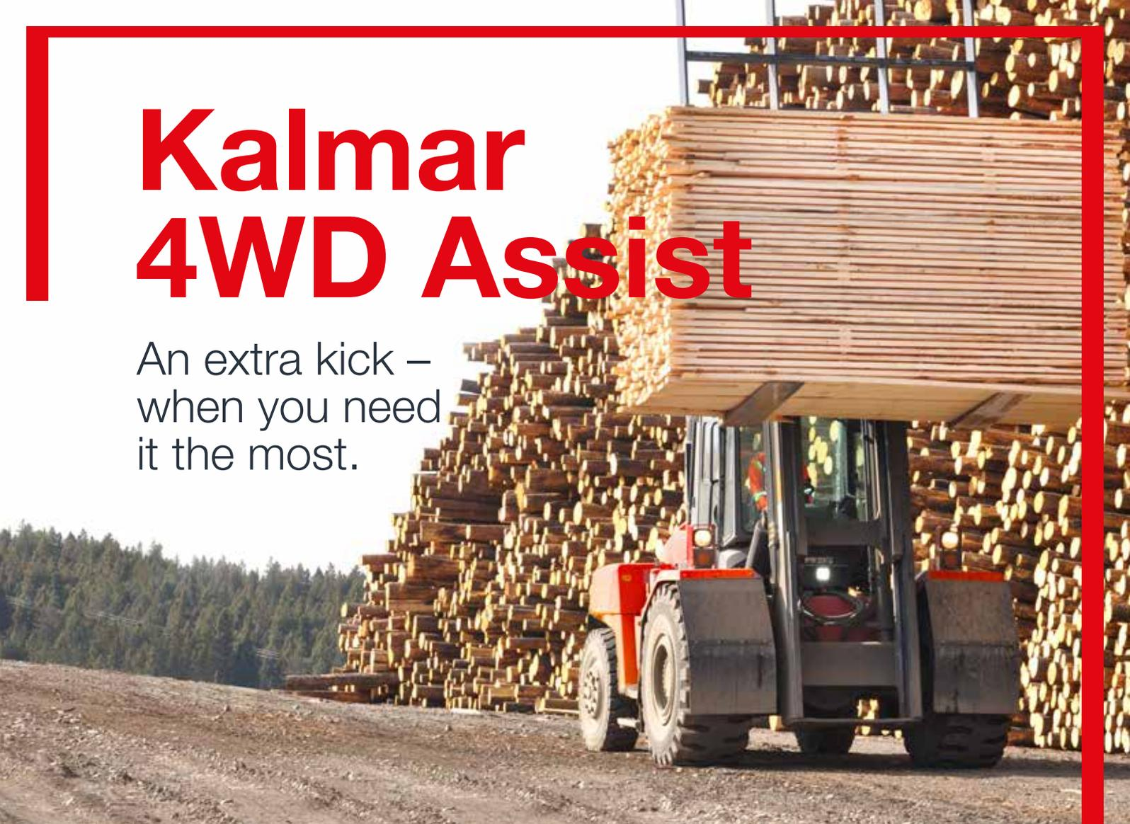
Working on snowy ground? A slippery surface at a sawmill? A muddy construction site? Then you know the frustration when your front wheels lose traction – just when you need the power the most. Kalmar's 4WD Assist option gives you that extra kick through a temporary four-wheel drive boost.
