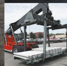
Machine details: This DRG450-60S5 reachstacker was delivered with two attachments. The first a tilling head with a safety clamp that grips the container while it is being titled and the second, hooks for lifting coils. It can lift loads of up to 45 tonnes.
